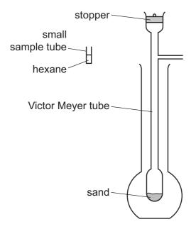
A small sample tube containing the hexane is inserted at the top of the Victor Meyer tube. The sample tube is small enough to fit inside the Victor Meyer tube and falls freely onto the hot sand below. The sand will cushion its fall so that the sample tube does not break. The stopper is then quickly replaced at the top of the Victor Meyer tube. The hot sand causes the hexane to vaporise and expel air contained in the Victor Meyer tube.
